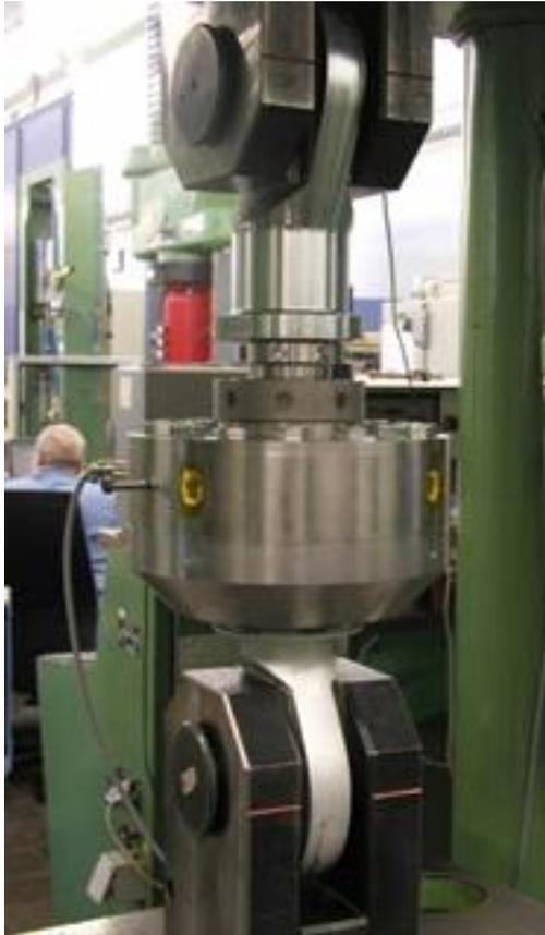
*Use of two knuckle eyes for calibration of a U10M with a maximum capacity of 500 kN*
