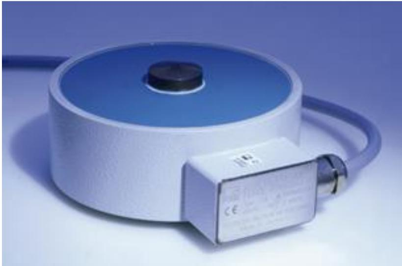
Transducers designed so they are only able to record forces in the pressure direction are generally equipped with a convex fitting for application of the load.
